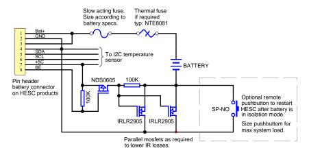
Figure A1: Battery Mosfet Isolation Circuit
